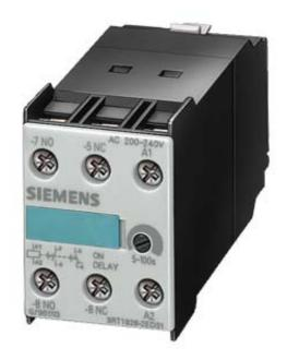
SOLID-STATE, TIME-DELAYED AUXILIARY SWITCH BLOCK SETTING RANGE 0.5 S...10 S AC 200...240 V, 1NO + 1NC, ON-DELAY, FOR MOUNTING ONTO CONTACTORS SIZE S0...S12
