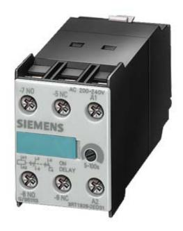
SOLID-STATE, TIME-DELAYED AUXILIARY SWITCH BLOCK SETTING RANGE 0.5 S...10 S AC 100...127 V, 1NO + 1NC, ON-DELAY, FOR MOUNTING ONTO CONTACTORS SIZE S0...S12
