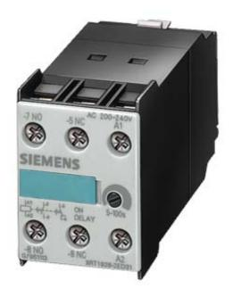
SOLID-STATE, TIME-DELAYED AUXILIARY SWITCH BLOCK SETTING RANGE 0.5 S...10 S, AC/DC 24 V, 1NO + 1NC, ON-DELAY, FOR MOUNTING ONTO CONTACTORS SIZE S0...S12
