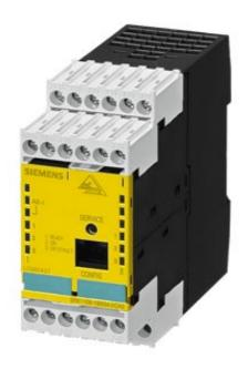
ASISAFE BASIC SAFETY MONITOR 2 F-RO, 2 ENABLING CIRCUITS, IP20, WITH SCREW-TYPE TERMINALS (REMOVABLE), SAFE OUTPUT RELAY RESPONSE TIME MAX. 50 MS, MONITOR TYPE 2, VERSION 3, APPLICABLE UP TO CATEGORY 4 (EN 954-1), UP TO PL E (EN ISO 13849-1), UP TO SIL 3 (IEC 61508), FOR AS-INTERFACE / AS-I SAFETY AT WORK
