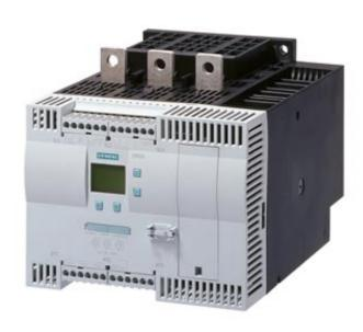
SIRIUS SOFT STARTER, VALUES WITH 400 V, 40 DEG., STANDARD: 250A, 132KW, INSIDE-DELTA CIRCUIT 3: 433A, 250KW, 200-460 V AC, 230 V AC, CAGE CLAMP TERMINALS
