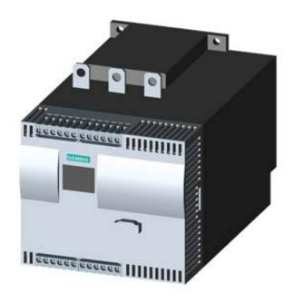
SIRIUS SOFT STARTER, VALUES WITH 400 V, 40 DEG., STANDARD: 113A, 55KW, INSIDE-DELTA CIRCUIT 3: 196A, 110KW, 200-460 V AC, 230 V AC, CAGE CLAMP TERMINALS
