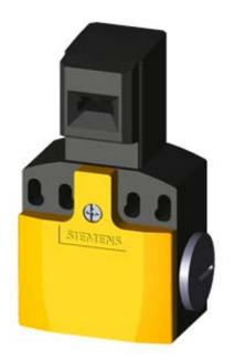
SAFETY POS. SWITCH W. SEPARATE ACTUATOR, PLASTIC ENCLOSURE, 50MM; 2X(M20X1.5) SLOW-ACTION CONTACTS 1NO+2NC 5 DIRECTIONS OF APPROACH THE MATCHING SEPARATE ACTUATOR 3SE5000-0AV0. IS TO BE ORDERED SEPARATELY
