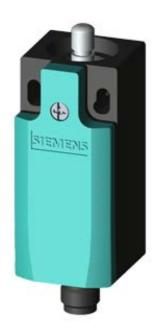
SIRIUS POSITION SWITCH; PLASTIC HOUSING ACC. TO EN50047, 31MM 1NO/2NC SNAP-ACTION CONTACTS W. M12 CONNECTOR,4-POLE MAX.250V AND 4A, 20E AND PE CONNECTED TEFLON PLUNGER
