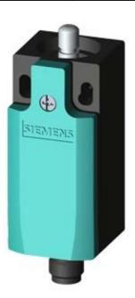
SIRIUS POSITION SWITCH; PLASTIC HOUSING ACC. TO EN50047, 31MM 1NO/2NC SLOW-ACTION CONTACTS W. M12 CONNECTOR,4-POLE MAX.250V AND 4A, 20E AND PE CONNECTED TEFLON PLUNGER
