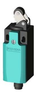
SIRIUS POSITION SWITCH; PLASTIC HOUSING ACC. TO EN50047, 31MM 1NO/1NC SNAP-ACTION CONTACTS INTEGRATED (NOT REPLACEABLE) W. M12 CONNECTOR, 4-POLE PIN ASSIGNMENT: PIN1=21, PIN2=22, PIN3=13,PIN4=14, MAX. 250V AND 4A ROLLER LEVER W. PLASTIC ROLLER 13MM
