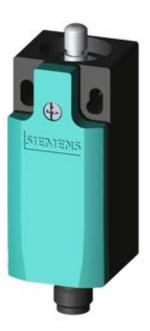
SIRIUS POSITION SWITCH; PLASTIC HOUSING ACC. TO EN50047, 31MM 1NO/1NC SLOW-ACTION CONTACTS W. M12 CONNECTOR,4-POLE PIN ASSIGNMENT: PIN1=21, PIN2=22, PIN3=13,PIN4=14, MAX.250V AND 4A, TEFLON PLUNGER
