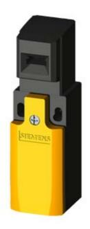
SAFETY POS. SWITCH W. SEPARATE ACTUATOR, PLASTIC ENCLOSURE, 31MM; 1X(M20X1.5) SLOW-ACTION CONTACTS 1NO+1NC, 5 DIRECTIONS OF APPROACH, THE MATCHING SEPARATE ACTUATOR 3SE5000-0AV0. IS TO BE ORDERED SEPARATELY
