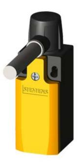
SIRIUS HINGED SWITCH PLASTIC HOUSING,31MM,EN50047 DEVICE CONNECTION 1X(M20X1.5) SNAP-ACTION CONTACTS 1NC/1NO INTEGR.,W. SOLID SHAFT D=10MM ACTUATING ANGLE 10 DEGR.
