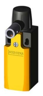
SIRIUS HINGED SWITCH PLASTIC HOUSING,31MM,EN50047 DEVICE CONNECTION 1X(M20X1.5) SNAP-ACTION CONTACTS 1NC/1NO INTEGR.,W. HOLLOW SHAFT D=8MM; ACTUATING ANGLE 10 DEGR.
