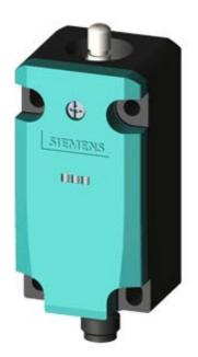
BASIC SWITCH FOR POSITION SWITCH 3SE51, METAL HOUSING 40MM TO EN50041,1NO/1NC SNAP-ACTION CONTACTS W. M12 CONNECTOR, 5-POLE, FIXED W. 2 LEDS, YELLOW/GREEN, 24V DC,
