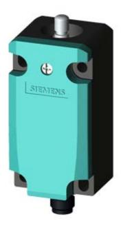
BASIC SWITCH FOR POSITION SWITCH 3SE51. METAL ENCLOSURE 40MM TO EN50041 DEVICE CONNECTION 1X (M20X1.5) W. M12 CONNECTOR, 5-POLE, FIXED 1NO/2NC SNAP-ACTION CONTACTS, (2NC AND PE CONNECTED) MAX. 24 V, 4A
