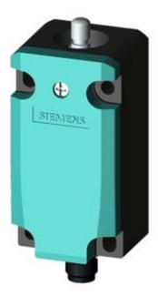
BASIC SWITCH FOR POSITION SWITCH 3SE51. METAL ENCLOSURE 40MM TO EN50041 DEVICE CONNECTION 1X (M20X1.5) W. M12 CONNECTOR, 5-POLE, FIXED 1NO/2NC SLOW-ACTION CONTACTS, (2NC AND PE CONNECTED) MAX. 24 V, 4A
