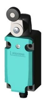
SIRIUS POSITION SWITCH METAL ENCLOSURE 40MM TO EN50041 1NO/ 1NC SNAP-ACTION CONTACTS W. M12 CONNECTOR, 5-POLE, FIXED PIN ASSIGNMENT: PIN1=21, PIN2=22, PIN3=13, PIN4=14, PIN5=PE ROTARY ACTUATOR RIGHT AND/ OR LEFT ADJUSTABLE,
