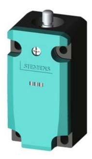
BASIC SWITCH FOR POSITION SWITCH 3SE51. METAL ENCLOSURE 40MM TO EN50041 W. 2 LEDS, YELL./GREEN, 24V DC, 1X(M20X1.5) 1NO/2NC SLOW-ACTION CONTACTS W/O ACTUATOR HEAD
