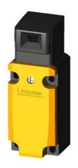
SAFETY POS. SWITCH W. SEPARATE ACTUATOR, METAL HOUSING,40MM, 1X(M20X1.5) SLOW-ACTION CONTACTS 1NO/2NC 5 DIRECTIONS OF APPROACH
