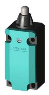
SIRIUS POSITION SWITCH METAL ENCLOSURE 40MM TO EN50041 DEVICE CONNECTION 1X (M20X1.5) 1NO/ 2NC SNAP-ACTION CONTACTS ROUNDED PLUNGER W. 3MM OVER- TRAVEL, STAINLESS STEEL PLUNGER
