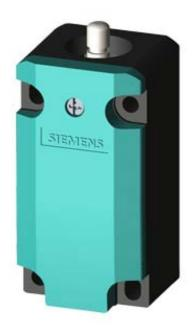
BASIC SWITCH FOR POSITION SWITCH 3SE51, METAL ENCLOSURE, ACC. TO EN50041 DEVICE CONNECTION 1X (M20X1.5) 1NO/2NC SNAP-ACTION CONTACTS W/O ACTUATOR HEAD
