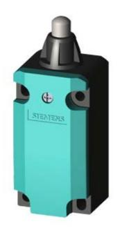
SIRIUS POSITION SWITCH METAL ENCLOSURE 40MM ACC. TO EN50041 DEVICE CONNECTION 1X (M20X1.5) 1NO/1NC SNAP-ACTION CONTACTS ROUNDED PLUNGER W. 3MM OVER- TRAVEL, STAINLESS STEEL PLUNGER
