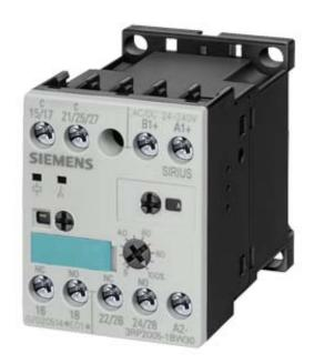
SOLID-STATE TIME-DELAY RELAY MULTI-FUNCTION, 8 FUNCTIONS 1 CHANGEOVER CONTACT AC/DC 24V, AC 200 TO 240V 0.05 S TO 100H WIDTH 45MM SCREW TERMINALS
