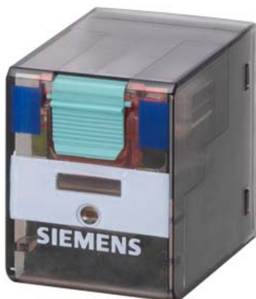
PLUG-IN RELAY, 3 CO CONTACTS, 24V AC, 10A, WIDTH 22.5MM
