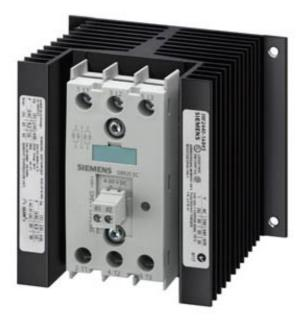
SEMI-CONDUCTOR CONTAC.3-PH.3RF2 AC51 40A 40 DEG. C 48-600V / 230V AC 2-PHASE CONTROLLED SCREW TERMINAL BLOCKING VOLTAGE 1200V
