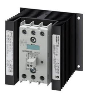
SEMI-CONDUCTOR CONTAC.3-PH.3RF2 AC51 30A 40 DEG. C 48-600V / 230V AC 3-PHASE CONTROLLED SCREW TERMINAL BLOCKING VOLTAGE 1200V
