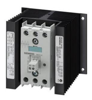
SEMI-CONDUCTOR CONTAC.3-PH.3RF2 AC51 30A 40 DEG. C 48-600V / 4-30V DC 3-PHASE CONTROLLED SCREW TERMINAL BLOCKING VOLTAGE 1200V
