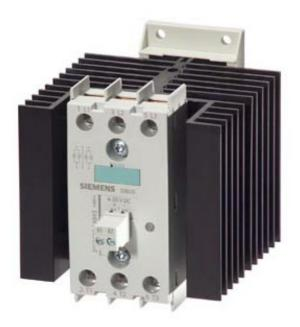
SEMI-CONDUCTOR CONTAC.3-PH.3RF2 AC51 30A 40 DEG. C 48-600V / 230V AC 2-PHASE CONTROLLED SCREW TERMINAL BLOCKING VOLTAGE 1200V
