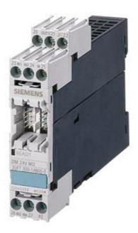
DIGITAL MODULE; 4 INPUTS AND 2 RELAY OUTPUTS; INPUT VOLTAGE DC 24V; MONOSTABLE RELAY OUTPUTS; MAXIMUM 2 DIGITAL MODULES PER BASIC UNIT 2
