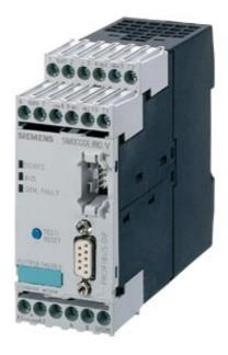
BASIC UNIT 2 SIMOCODE PRO V; PROFIBUS DP INTERFACE 12 MBIT/S, RS485; 4I/30 FREELY PARAMETERIZABLE; US: DC 24V; THERMISTOR MOTOR PROTECTION; RELAY OUTPUTS MONOSTABLE; EXPANDABLE BY EXPANSION MODULES
