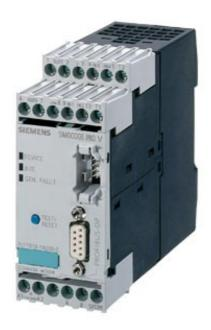
BASIC UNIT 2 SIMOCODE PRO V; PROFIBUS DP INTERFACE 12 MBIT/S, RS485; 41/30 FREELY PARAMETERIZABLE; US: AC/DC 110-240V; INPUT F. THERMISTOR MOTOR PROTECTION; RELAY OUTPUTS MONOSTABLE; EXPANDABLE BY EXPANSION MODULES
