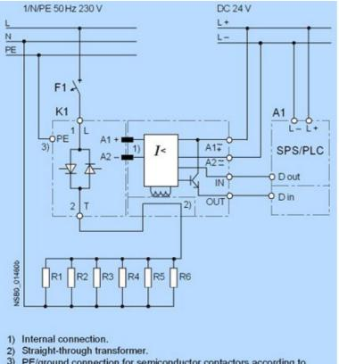
PE/ground connection for semiconductor contactors according to installation regulations.
