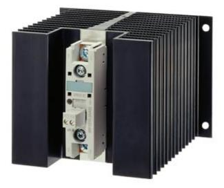
SEMI-COND. CONTACTOR 3RF2,1-PH. AC 51 70A/AC15 27.5A 40 DEG. C 24-230 V / 24 V DC INSTANTANEOUS SWITCHING
