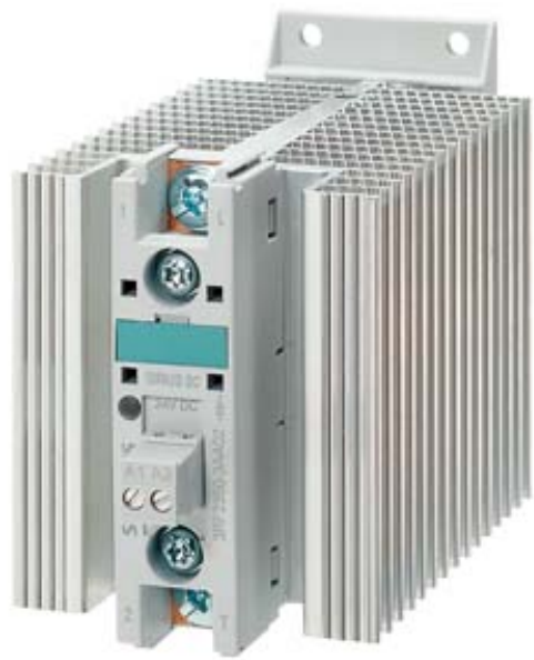
SEMI-COND. CONTACTOR 3RF2,1-PH. AC 51 50 A 40 DEGREES C 24-230 V / 24 V DC RING TERMINAL
