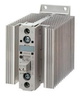
SEMI-COND. CONTACTOR 3RF2,1-PH. AC 51 50A / AC15 25A 40 DEG. C 24-230 V / 110-230 V AC INSTANTANEOUS SWITCHING
