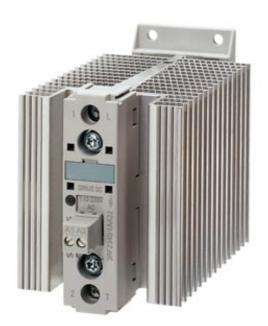
SEMI-COND. CONTACTOR 3RF2,1-PH. AC 51 50A / AC15 25A 40 DEG. C 48-460 V / 24 V DC INSTANTANEOUS SWITCHING
