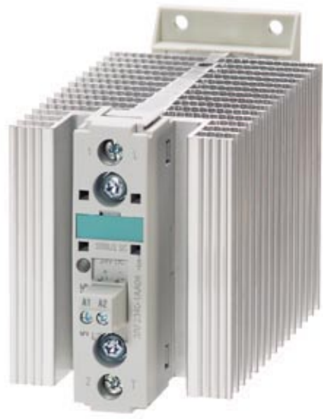
SEMI-COND. CONTACTOR 3RF2,1-PH. AC 51 40 A 40 DEGREES C 48-460 V / 110-230 V AC SCREW TERMINAL
