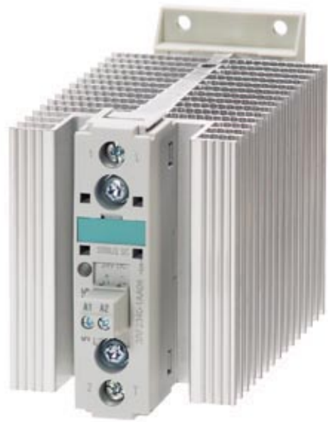
SEMI-COND. CONTACTOR 3RF2,1-PH. AC 51 40 A 40 DEGREES C 48-600 V / 24 V DC SCREW TERMINAL
