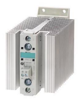
SEMI-COND. CONTACTOR 3RF2,1-PH. AC 51 40A / AC15 20A 40 DEG. C 48-600 V / 110-230 V AC INSTANTANEOUS SWITCHING
