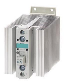
SEMI-COND. CONTACTOR 3RF2,1-PH. AC 51 40A / AC15 20A 40 DEG. C 48-460 V / 110-230 V AC INSTANTANEOUS SWITCHING
