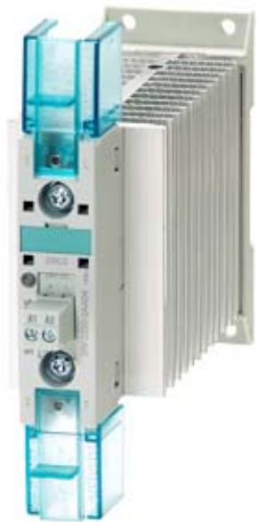
SEMI-COND. CONTACTOR 3RF2,1-PH. AC 51 30 A 40 DEGREES C 24-230 V / 110-230 V AC RING TERMINAL
