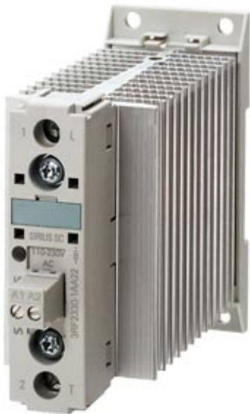
SEMI-COND. CONTACTOR 3RF2,1-PH. AC 51 30 A 40 DEGREES C 48-600 V / 110-230 V AC SCREW TERMINAL
