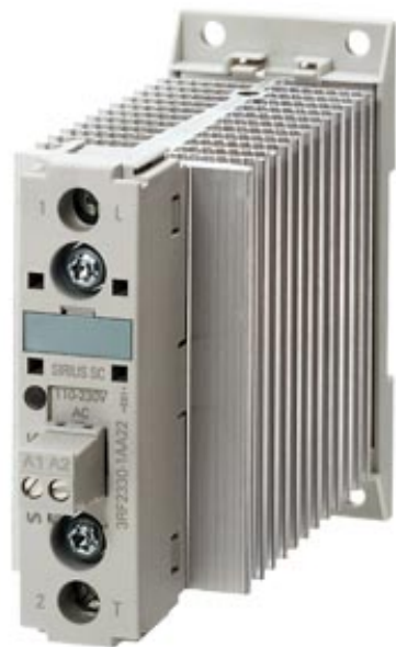
SEMI-COND. CONTACTOR 3RF2,1-PH. AC 51 30 A 40 DEGREES C 24-230 V / 110-230 V AC SCREW TERMINAL
