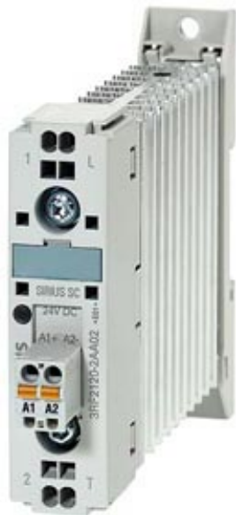
SEMI-COND. CONTACTOR 3RF2,1-PH. AC 51 20 A 40 DEGREES C 48-460 V / 110-230 V AC SPRING-LOADED TERMINAL
