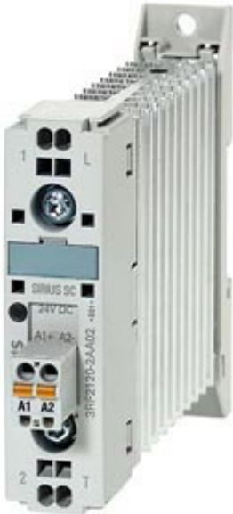
SEMI-COND. CONTACTOR 3RF2,1-PH. AC 51 20 A 40 DEGREES C 24-230 V / 110-230 V AC SPRING-LOADED TERMINAL
