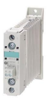
SEMI-COND. CONTACTOR 3RF2,1-PH. AC 51 20 A 40 DEGREES C 48-460 V / 110-230 V AC SHORT-CIRC. RESIST. WITH B-MCB
