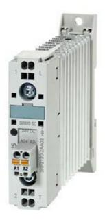
SEMI-COND. CONTACTOR 3RF2,1-PH. AC 51 10 A 40 DEGREES C 48-600 V / 24 V DC SPRING-LOADED TERMINAL
