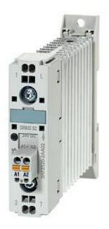
SEMI-COND. CONTACTOR 3RF2, 1-PH AC 51 10 A 40 DEGREES C 24-230 V / 24 V DC SPRING-LOADED TERMINAL
