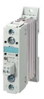
SEMI-COND. CONTACTOR 3RF2, 1-PH AC 51 10 A / AC15 6A 40 DEG. C 48-600 V / 110-230 V AC INSTANTANEOUS SWITCHING
